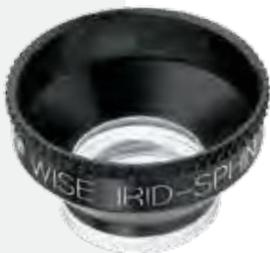
This lens features a 9mm diameter, 103D magnifying lens strategically aligned to optimize small spot laser delivery. Laser power density at the iris is 2.7 times greater than with an Abraham lens and 6.9 times greater than with a flat lens. Increases treatment efficiency with less energy and shorter burn duration, even on thick brown or light blue irises. Useful with Argon/Diode or Nd:YAG lasers.
