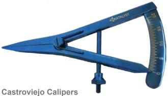
Measures from 0mm to 20mm in .5mm increments with scale reading on one side.
