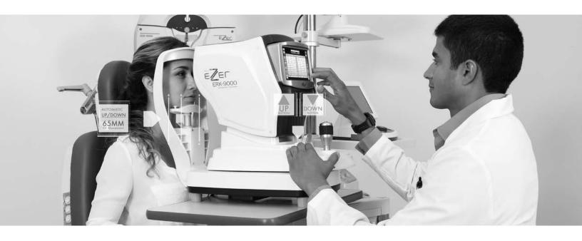
The ERK-9000 is comfortable for patients and convenient for operators. With the simple press of a button you can set the chin rest and measuring point. The ERK-9000 allows for 65mm of movement.
